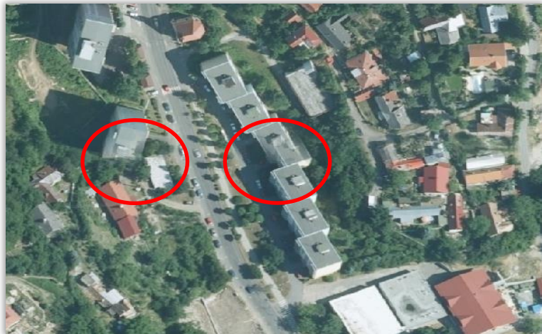
Example of errors resulting from incorrect alignment of seamlines
