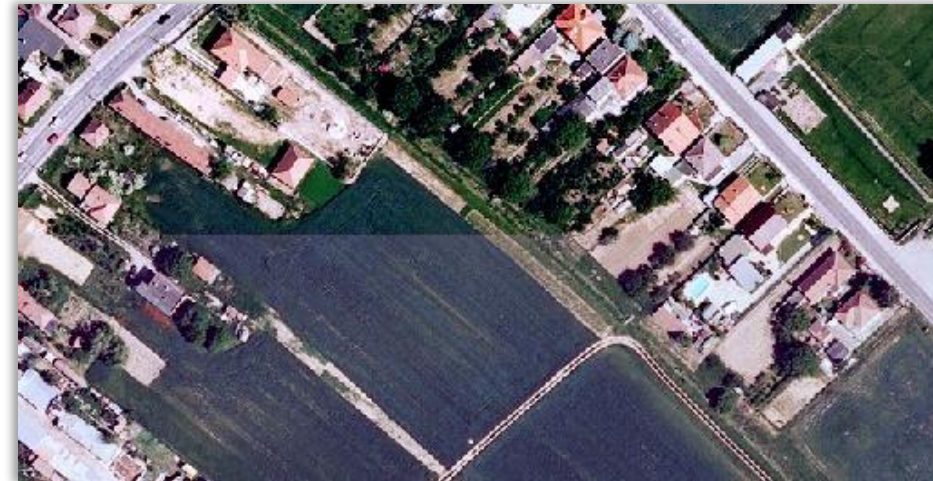
Example incorrect color properties of the image around the seamlines
