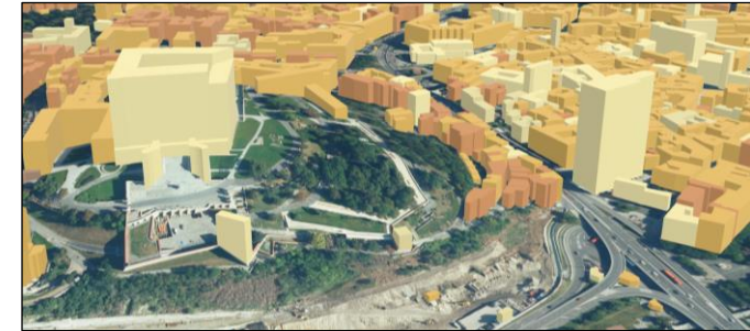
LoD 2 – shape of the object with an emphasis on the shape of the roof covering
